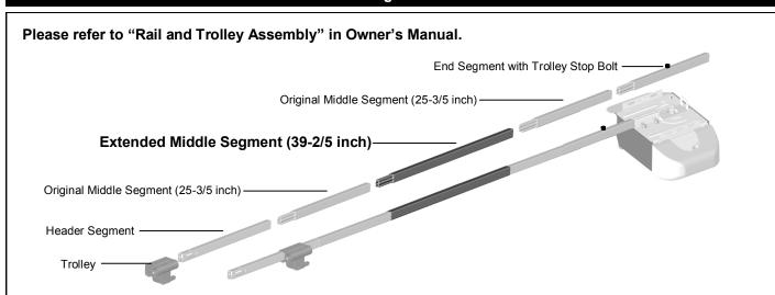
Replace ONE of the original rail Middle Segment with the "Extended Rail Segment" in the middle of rail assembly.
